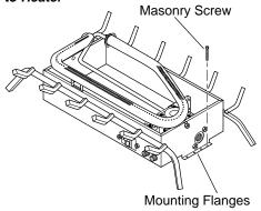
Figure 12 - Attaching Base Assembly to Fireplace Floor
